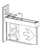
Secure the exit sign to the wall bracket by tightening the screws.
